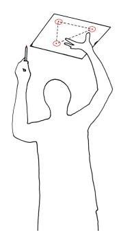
Bohren / Drill Trapano / Foret ø 6,0 mm
