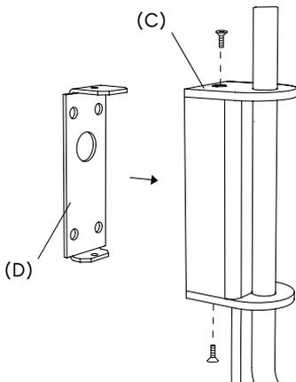
2. Remove the wall mounting (D) by unscrewing two screws from the lamp body (C).
