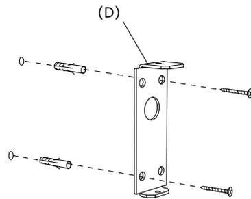
3. Mount the wall mounting to the wall with two appropriate screws and plugs. Always use correct screws and plugs for the mounting surface.
