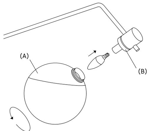
5. Insert the light bulb then gently mount the diffuser screwing it back to the metal ring.
