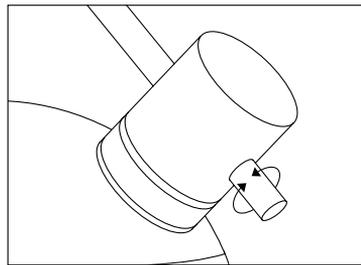
Rotate dimmer switch to adjust light intensity.
