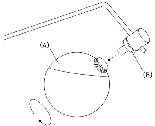
1. Unscrew the diffuser (A) while holding the metal ring (B).
